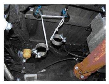
Slide Mufflex Retro-Fit muffler in place using the rear hanger for alignment.
